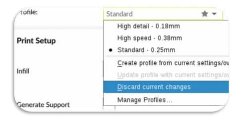
**High Detail** - Designed to give greater detail and finer objects. This will have a smaller layer height, which will make each layer thinner, so that curves seem more natural and walls seem less noticeable. This setting will also require more layers to be laid down, increasing overall print time.
