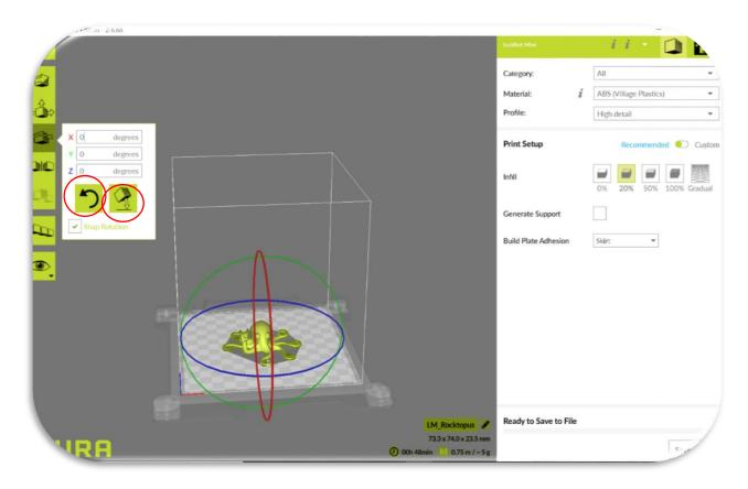
**Lay Flat** - The Lay Flat button will ensure that the flat portion of your print is securely attached to the bed. It is highly recommended to use this option after rotating your model in the Z direction, as it will help prevent adhesion issues during the print.
