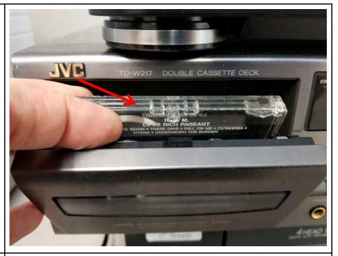
Close the door on the cassette deck. Couple of things to note here. The first thing you should do is rewind the tape marked by two left facing triangles. Once the tape is rewound, you can press **COUNTER RESET** to put the counter back at 00:00 time code. Lastly, ensure that the **REVERSE MODE** switch is set to the middle for one automatic palyback of the reserve side of the tape. This will ensure that you don't need to flip the cassette once Side A has finished.
