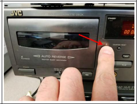
Load up an audio cassette, ensuring that the tape side is on the bottom when inserting the cassette into the cassette deck. Side A of the cassette should be facing you.
