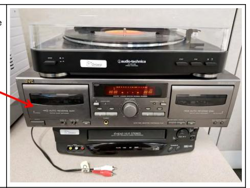
Using the 3-way coupler adapter/extender, make sure that the white cables align with each other as well as the red cables. The white audio cable is for left channel audio while the red cable represents the right channel audio.
