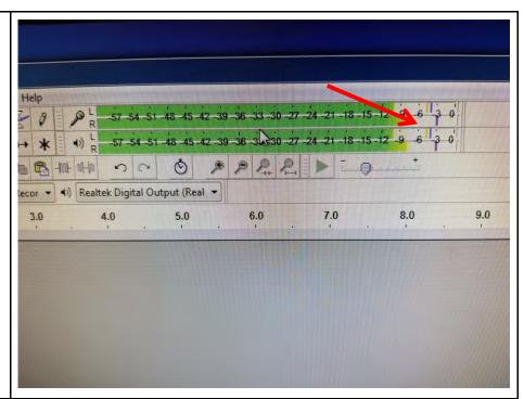
Let's start capturing in Audacity. Click on the **Record** button (red round circle). Note the nice clean waveform being generated as the signal is constrained to 0.5 never really hitting the top of 1.0 (which will produce noticeable clipping).
