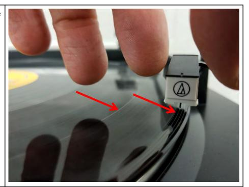
Press the **UP / DOWN arrows** button once again to lower the tonearm into position.
