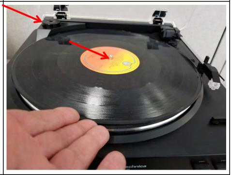
Remove the protective plastic shielding that is protecting the turntable cartridge / needle.
