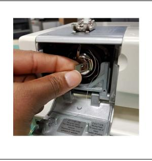
Hold the bobbin case by the latch with the index finger and thumb of the left hand.
