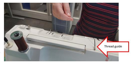
hook the thread into the (4) Needle Holder Thread Guide before threading the needle.
