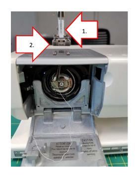
Raise the needle (1) by turning the balance wheel on the side of the machine. Raise the presser foot (2), by lifting the presser foot lever which is located on the back of the machine.
