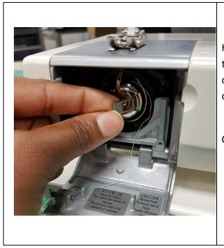
Hold the bobbin case by the latch with the index finger and thumb of the left hand. Insert so that the finger of the bobbin case points upwards, engaging in the notch of the hook race cover.
