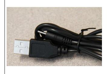
Attach the USB end to the computer or a USB charger and the other end into the top of the pen
