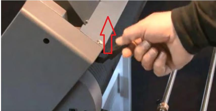
Lock the lever on the back right side of the machine, by pulling it upward.
