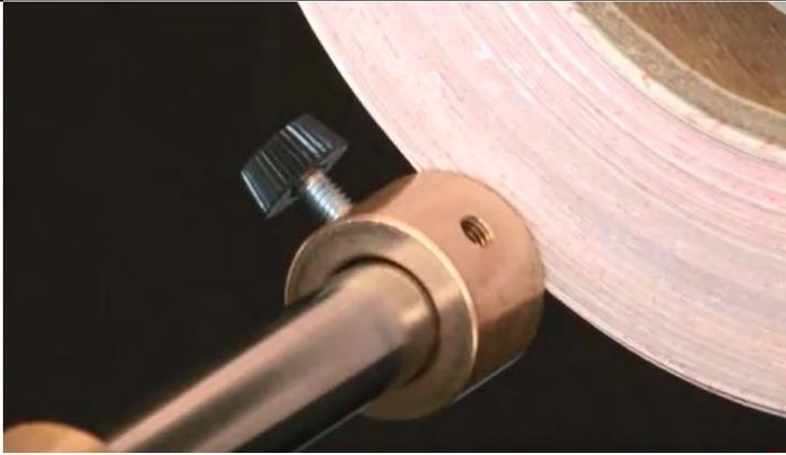
Make sure it is in position with the stoppers, so the roll of paper doesn't slide.
