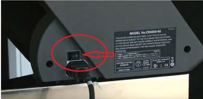
Turn the machine on using the power button located on the left side.
