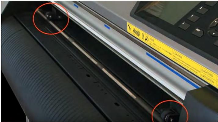
Move the roller guides to rest on the edge of each side of the vinyl.
