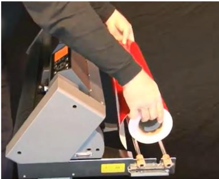
Unlock the lever down to load the paper.
