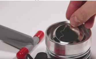
10.Replace Upper Die with the black "X" on top. Turn the black "X" counter clockwise, so that it becomes free from the ridges on the top of Upper Die.
