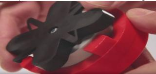
7. Slide the complete die into the machine, from left to right, until it is directly below the handle.
