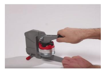
12. Slide the complete die to the left and out of the machine. Lift off Upper Die and remove your button.
