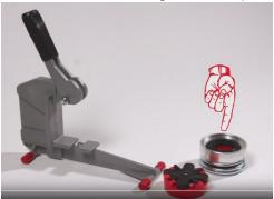
2. With its edges facing down, put the shell into the Pickup Die on top of the black ring.
