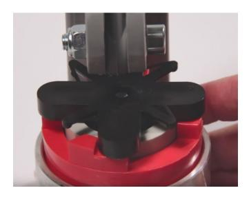
Pull the handle down until it will go no further (approximately halfway down). Use of extreme force is not necessary. After that slide the whole die to the left, and out of the machine.
