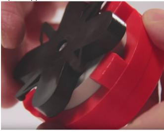
11.Slide the complete die into the machine again, from left to right, until it is directly under the handle. Now pull the handle down until it will go no further.
