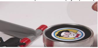
6. Place Upper Die on top of Pickup Die, with its black "X" facing up. Make sure that the black "X" is turned to its highest position, by lifting it and turning it clockwise, so that the wider arm, is resting on top of the black mark on the red ring.
