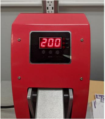
Press the middle button to see the temperature it needs to heat up to. Most of the time this should be "330".
