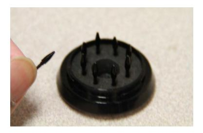
e) Push the new nib into the pen until its firmly in. Put the pen holder back together.
