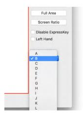
k) After, you can select which other keys need to be pressed. For the previous undo example, you would select command. More than one key can be selected, for example if you wanted to add Shift + Command + Z, you would need to check both Command and Shift. Now pressing the 3<sup>rd</sup> hotkey will simulate pressing Command+Shift+Z.
