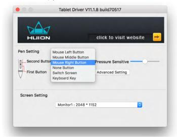
f) To change the Pressure Sensitivity, move the slider to left to make it less sensitive or right for more sensitive.
