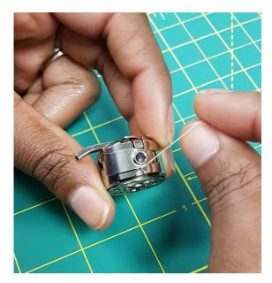
When the end of the thread is pulled, the bobbin should turn clockwise, in the direction of the arrow.
