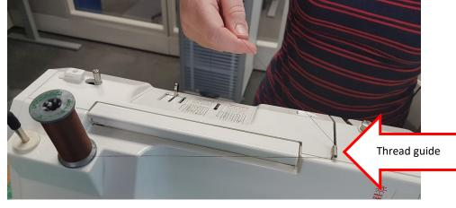
Bring the thread down through the channel at the front of the machine, and then loop it into the Guide Hook as you pull it upwards to the Take Up Lever. Once hooked into the take up leaver, pull the thread down towards the presser foot and then hook the thread into the Needle Holder Thread Guide before threading the needle.
