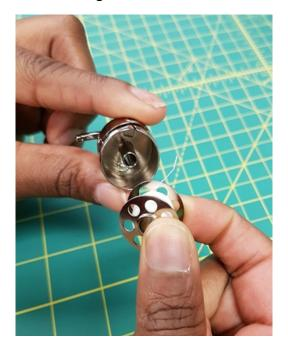
Take the thread anticlockwise to the slot
