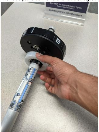
10. Place the new Paper Roll onto the Holder NOTE: Make sure the edge of the paper is facing forward (toward you)
