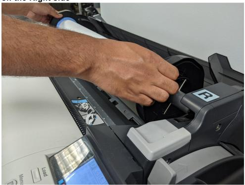
14. Start feeding the paper into the printer until the machine catches it
