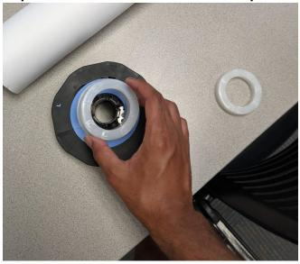
12. Place the Left Holder Stopper onto the Roll Holder until it's firm against the paper and re-lock it
