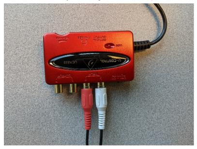
Make sure both cables are in the input slots and then plug the USB end of the capture device into the laptop.
