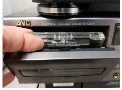
Close the door on the cassette deck. Couple of things to note here. The first thing you should do is rewind the tape marked by **two left facing triangles**. Once the tape is rewound, you can press **COUNTER RESET** to put the counter back at 00:00 time code. Lastly, ensure that the **REVERSE MODE** switch is set to the middle for one automatic playback of the reserve side of the tape. This will ensure that you don't need to flip the cassette once Side A has finished.
