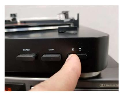
Position the cartridge to where you want to start playback of the record. Each song is separated and denoted by a wider groove or space on the record surface.
