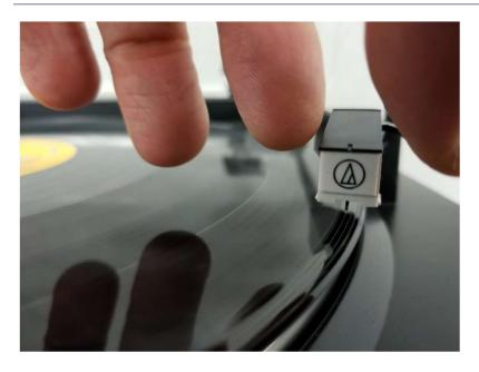
Press the **UP / DOWN arrows** button once again to lower the tonearm into position.
