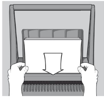
**3C** Punch pages by pulling handle down. Then lift the handle back to the vertical position and remove the punched sheets. Note: To prevent jams do not attempt to punch more than two cover sheets at a time.
