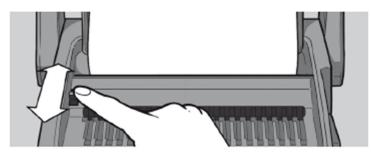
**3B** Load pages into slot. You can punch 2 cover sheets or up to 20 sheets of paper
