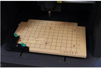
Once clear, remove the screws for the Smart Clamp and lift it off the corner.
