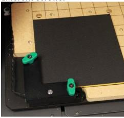
For the secondary clamps, take one of the long blocks with a hole in the middle and rest it on one of the step blocks as shown below.
