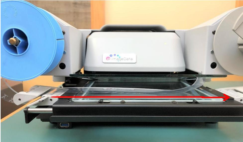
6. Feed the film into the right guide roller, weaving under the roller and around the right edge.
