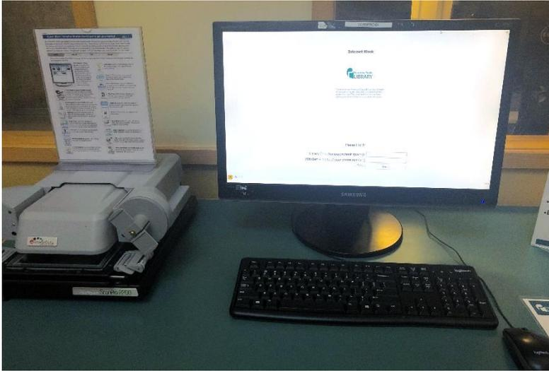
2. Turn the microfilm scanner on using the switch located on the right-hand side at the back of the machine.
