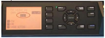
4. Hold down the blue ENTER button and if you're using Heat Transfer Vinyl, Press 1 and if you're using Sign Vinyl, Press 2
