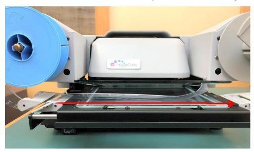
6. Feed the film into the right guide roller, weaving under the roller and around the right edge.
